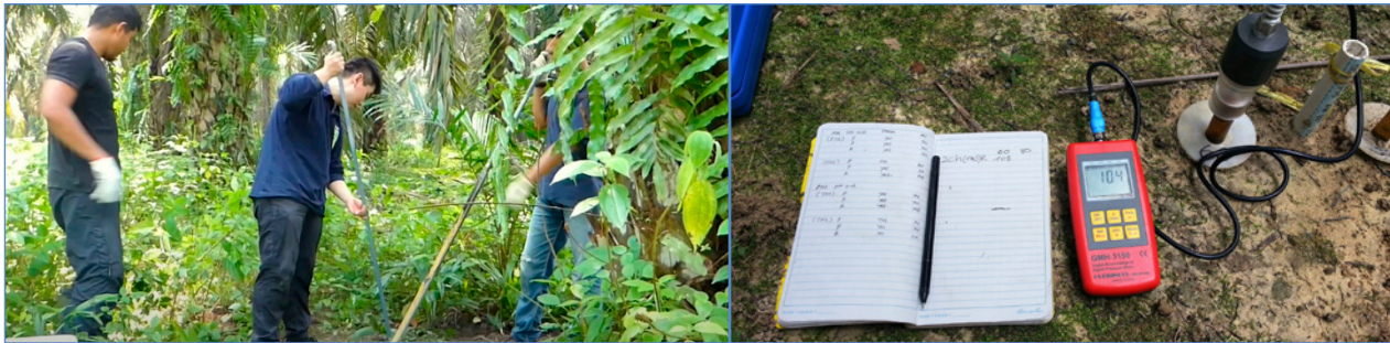
Picture 4. Installation of suction cup lysimeters at 1.5 m depth and tensiometers at 0.3 m and 0.6 m depths in each management zone per replicate plot.
