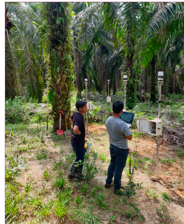
Picture 19. Measurement of below-canopy micrometeorology in PTPN6 oil palm plantation.
