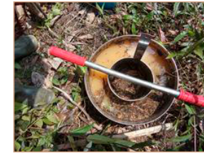
Picture 38. Infiltration measurements using double-ring infiltrometer. (Picture credit: A03-Landscape Assessment team).
